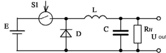
Figure-17. Converter circuit with a diode switch.
