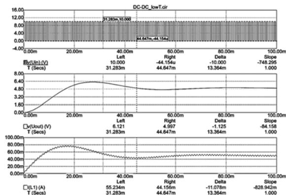
**Figure-21.** Voltage and current waveforms of a down DC-DC-converter with transistor switches.
