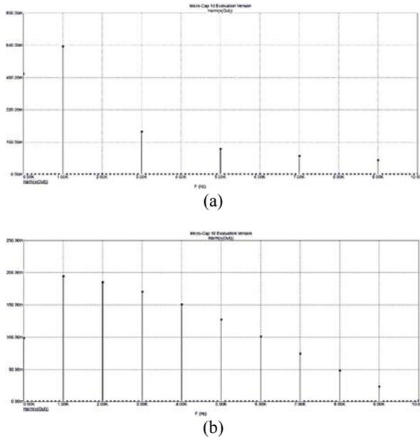
**Figure-3.** Unipolar pulse sequence spectra with the relative pulse duration  $Q=2$  (a) and  $Q=10$  (b).
