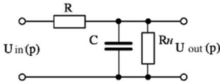
Figure-8. The LPF with the resistance load  $R_H$ .
