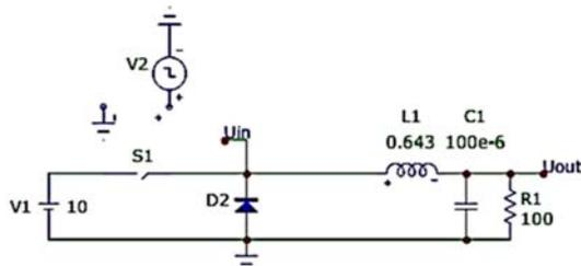
Figure-18. The circuit modeling of a down DC-DC-converter with a diode switch.
