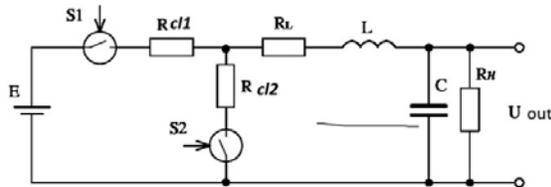
Figure-16. The analog circuit of a converter.
