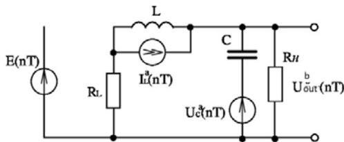
Figure-15. Circuit condition in phase "b".
