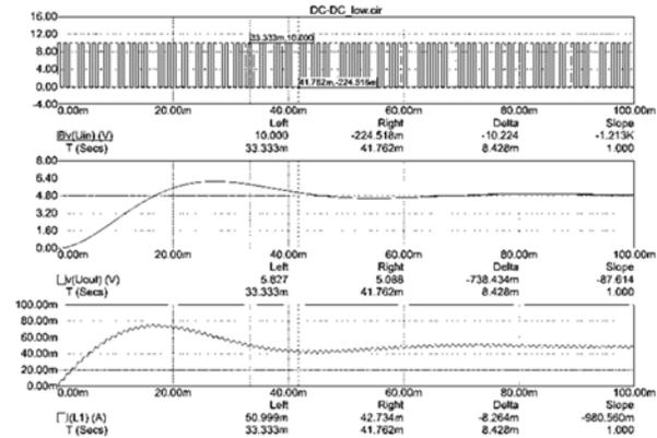
Figure-19. Voltage and current waveforms in the circuit of a down DC-DC-converter with a diode switch.
