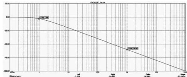
**Figure-6.** The AFR low pass filter of the first order with a cutoff, equal to 1Hz.
