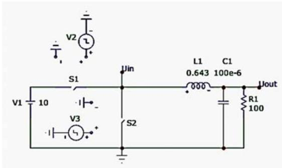
**Figure-20.** The circuit modeling of a down DC-DC-converter with transistor switches.
