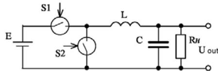
**Figure-11.** The circuit of a down pulse DC-DC-converter based on two electronic switches.
