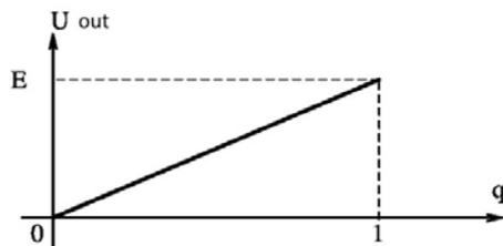
**Figure-13.** The regulating characteristic of a down DC-DC-converter.
