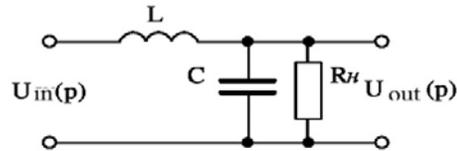
Figure-9. LPF circuit on a RLC-circuit basis.
